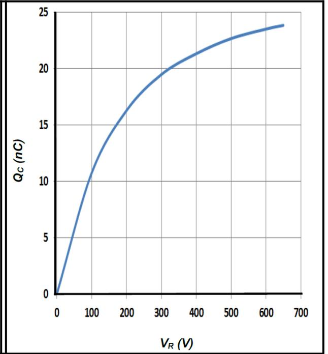
Figure 4. Total Capacitive Charge vs. Reverse Voltage
