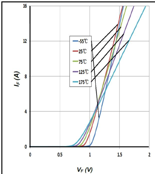
Figure 1. Forward Characteristics
