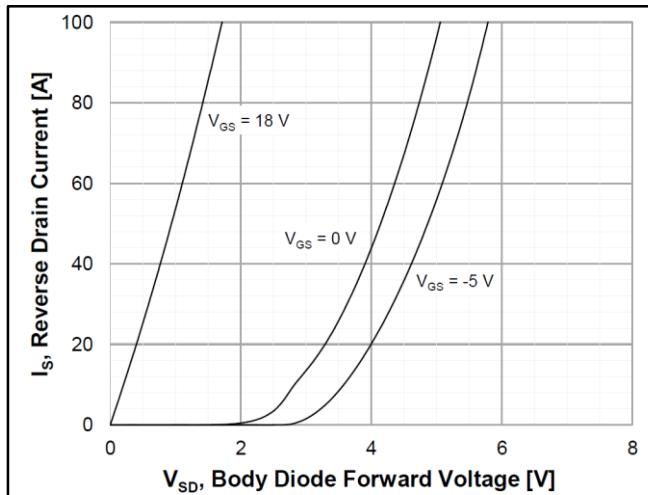
Figure 6. Body Diode Characteristics at  $-40\text{ }^{\circ}\text{C}$
