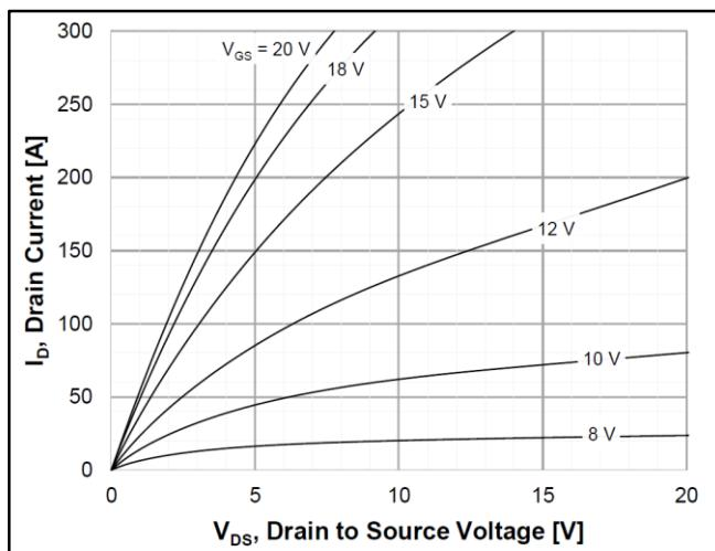
Figure 2. Output Characteristics  $T_J = 25\text{ }^{\circ}\text{C}$
