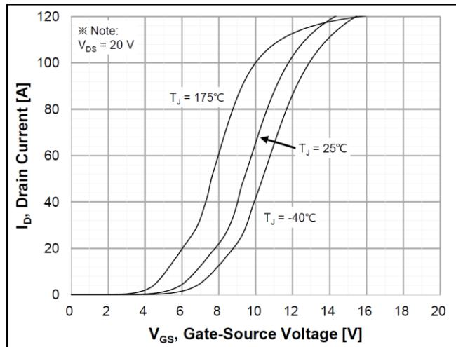
Figure 5. Transfer Characteristics for Various Junction Temperatures
