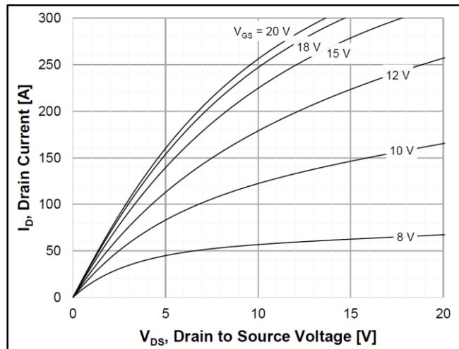
Figure 3. Output Characteristics  $T_J = 175\text{ }^{\circ}\text{C}$
