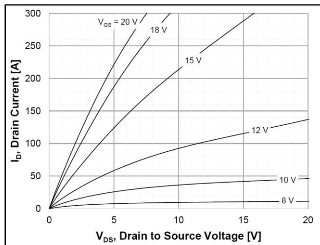
Figure 1. Output Characteristics  $T_J = -40\text{ }^{\circ}\text{C}$
