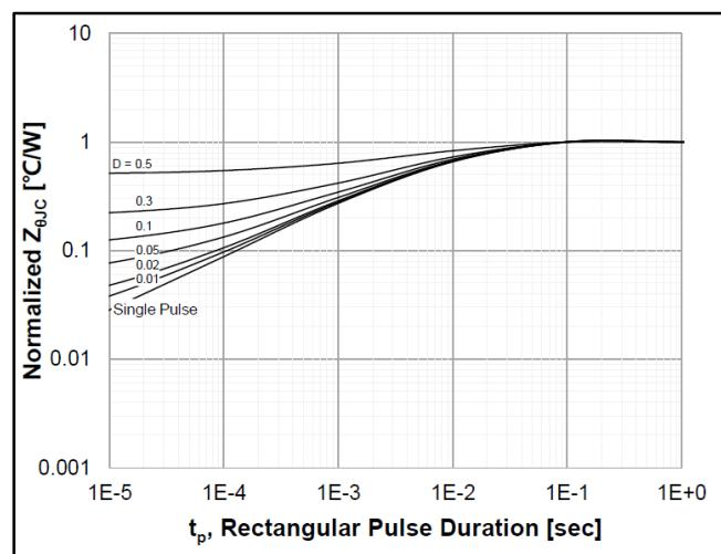
**Figure 19. Transient Thermal Impedance (Junction - Case)**
