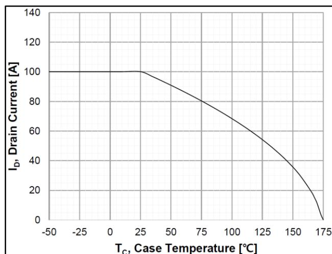
**Figure 13. Continuous Drain Current Derating vs. Case Temperature**
