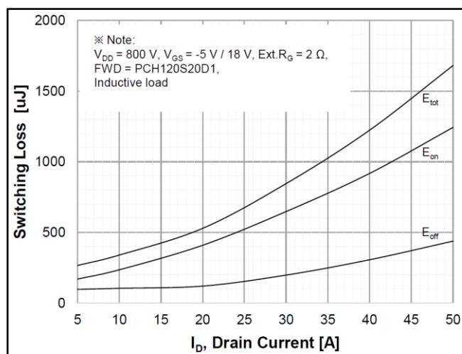
**Figure 15. Switching Losses vs. Drain Current**
